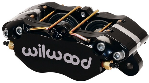
This brake kit uses Wilwood Dynapro 4 piston callipers with dust boots.
