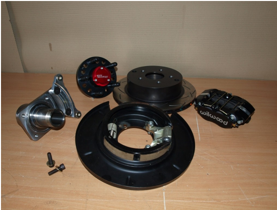
The kit is supplied with new Genuine OEM parking brake back plates, shoes and fittings
