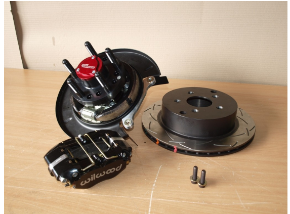
Genuine DBA Club Spec 4000 Series Rotors are CNC Milled to fit exactly with your choice of wheel stud pattern.
